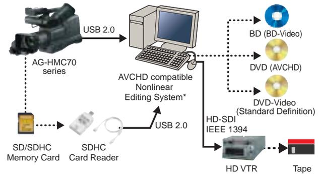
The AG-HMC70 series can be connected to an AVCHD nonlinear editing system by means of the USB interface or an SDHC card reader. This reduces production time by allowing high-speed data transfers without the need for digitizing.
