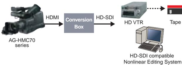
By using an HDMI/HD-SDI conversion box to convert data to an uncompressed HD stream, the AG-HMC70 series can be linked to existing linear/non-linear HD production environments using the DVCPRO HD format.
